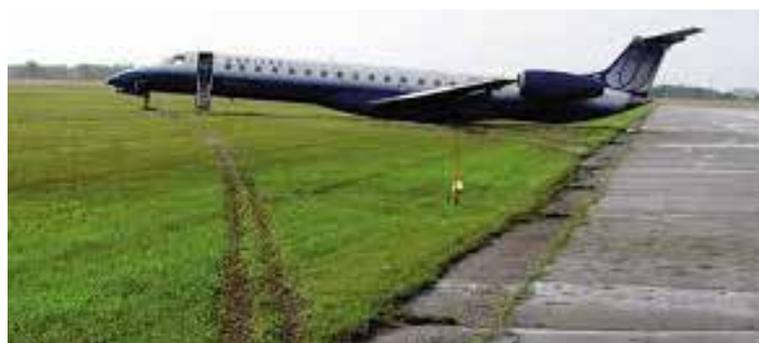
Embraer 145 runway excursion caused by unstabilized approach and improper braking technique during heavy rain.
